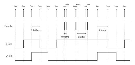
Fig. 2: Typical microprinter motor control signals
