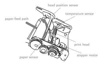
Fig. 1: Physical structure of the microprinter example
